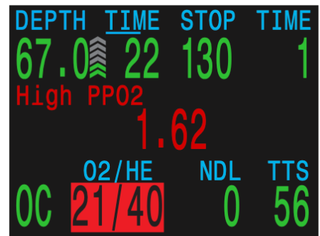
Sample "High PPO2" Persistent Notification
