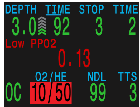
Sample "Low PPO2" Persistent Notification
